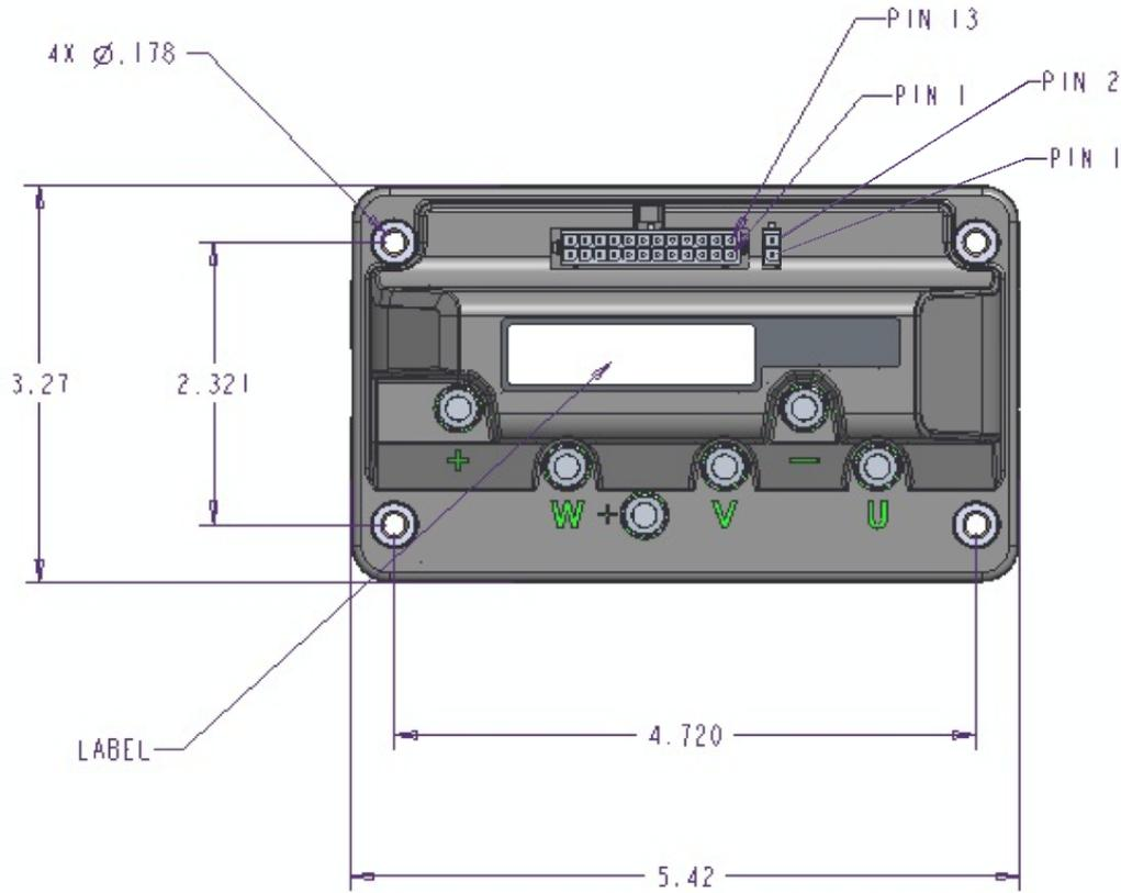
Motor and power connections should be made with properly sized wires and terminals, torqued to about 40-45 inch-pounds.
