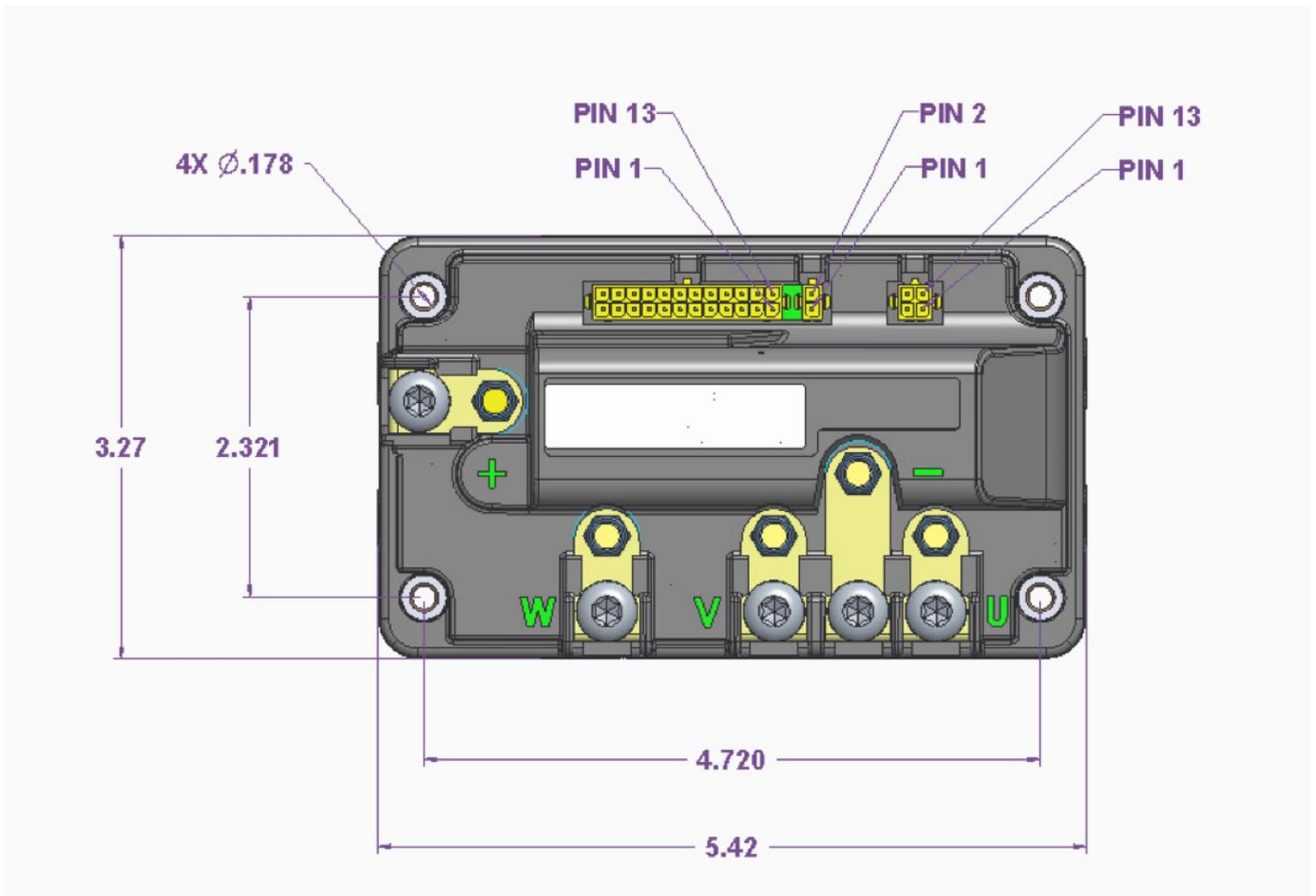
Motor and power connections should be made with properly sized wires and terminals, torqued to about 40-45 inch-pounds.
