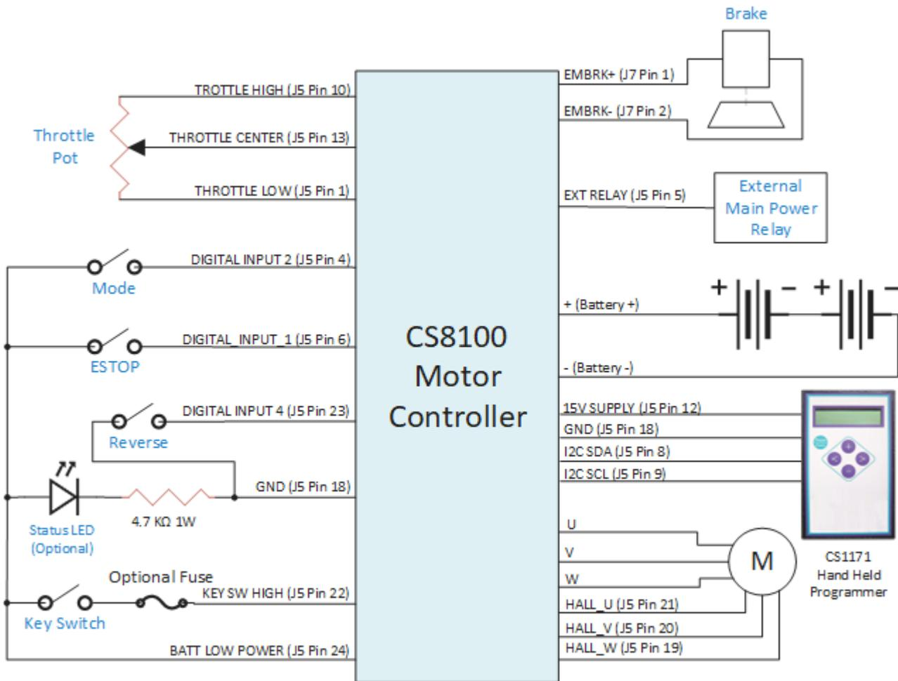
NOTE: The Configuration shown is for a BLDC motor. For a brushed motor the hall sensors are not used and only W & U or W & V are used for the motor leads.
